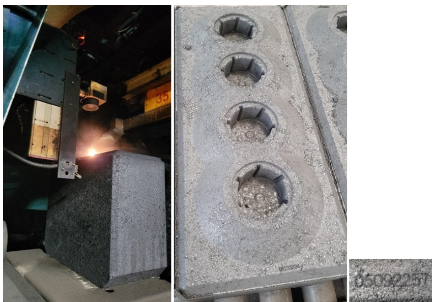
Figure 16. New laser marking device. Left: Laser. Right: Anode top face.
